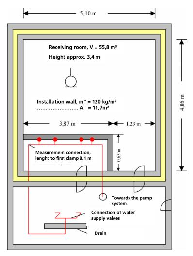
Section of test facility for water supply valves
