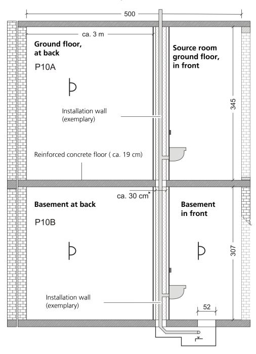
Vertical section of the test facility (dimensions in cm)
