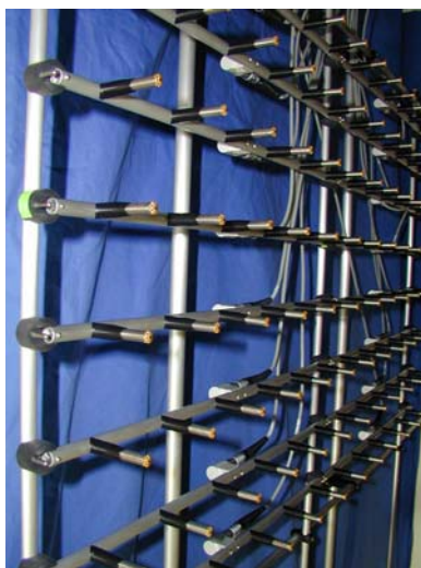
96 high-precision microphones combined on an array and connected to an analyser.
